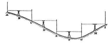
Let it be required to know the difference of level between the points A and I. The spirit level is set up at a point B, and the staff at A, and when, by the mechanical means previously spoken of, the spirit-level is brought truly horizontal, on looking through the telescope attached to it, the line of sight will be the dotted line towards the staff at A,
